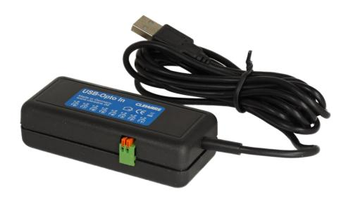
To interface digital input supplied in the range 4V to 24V the "USB-Opto In" is an easy way to go. The signals are connected with the USB device using professional clamp contacts, no screwing or soldering, nor opening the housing is required. The applied voltage is converted to a digital value using very robust military opto coupler (4N35M) and transferred to the computer. Up to eight independent channels are available.
